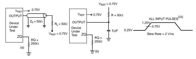
Note: 22. Unless otherwise noted, test conditions assume signal transition time of 2V/ns, timing reference levels of 0.75V, V<sub>REF</sub> = 0.75V, RQ = 250Ω, V<sub>DDQ</sub> = 1.5V, input pulse levels of 0.25V to 1.25V, and output loading of the specified I<sub>QL</sub>/I<sub>QH</sub> and load capacitance shown in (a) of AC Test Loads.
